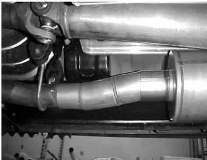
INSTALL HEADPIPE #A USING CLAMP #6 TO ATTACH IT TO THE STOCK HEADPIPE
