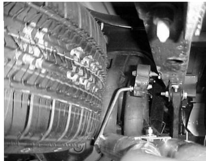
INSTALL DRIVERSIDE TAILPIPE #C TO OUTLET OF MUFFLER AND INSERT WELDED HANGER INTO RUBBER GROMMET. ATTACH TO MUFFLER WITH CLAMP #F. DRIVERSIDE TAILPIPE #C BRACKET SHOULD BE ON TOP OF TAILPIPE #D BRACKET. BOLT TAILPIPES TOGETHER USING BOLT KIT #I. DO NOT TIGHTEN UNTIL SYSTEM IS POSITIONED WITH 1" CLEARANCE FROM FRAME AND SHOCKS.
