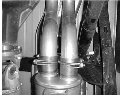
INSTALL PASSENGER TAILPIPE #D IN THE REAR OF THE MUFFLER. USE CLAMP # 6 TO ATTACH PASSENGER TAILPIPE TO. DO NOT TIGHTEN.
